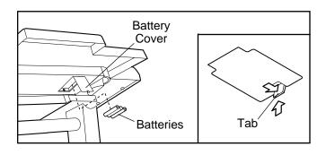
negative (-) ends of the batteries are touching the springs in the battery compartment. Close the battery cover, push up on the battery cover tab, and then push the tab forward as shown in the inset drawing. Be sure that the tab locks into place.
